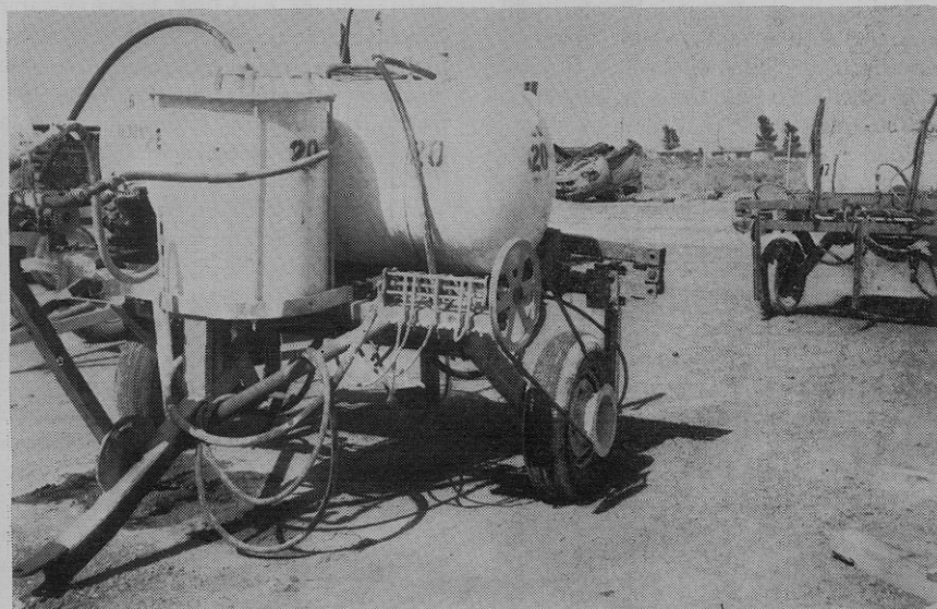
Figure 6. Rig for injecting anhydrous ammonia and phosphoric acid in soil
